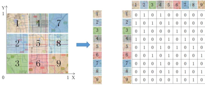
Figure 1. An illustration of how we get the adjacency matrix. In the left panel, the area [0, 1] \times [0, 1] is divided into 3 \times 3 = 9 equally sized rectangle regions. The right panel shows the corresponding adjacency matrix for these nine regions. We define two regions to be adjacent to each other if they share one common edge.
