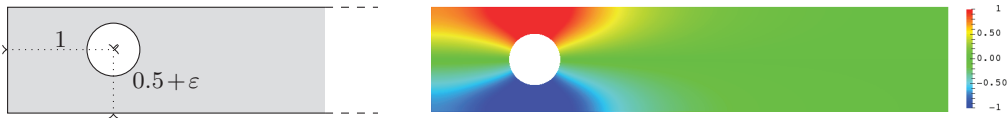
FIG. 7.5. Left: geometry of \Omega_+^\varepsilon . Right: real part of a trapped mode for \varepsilon = 0 and k^0 := \sqrt{\lambda^0} \approx 2.7403 .
