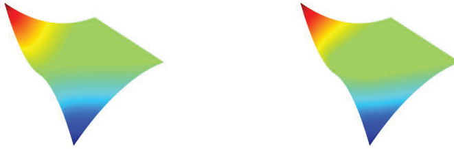
FIG. 5.7. The numerical solution for Example 8 on a grid of h=0.0078 (grid size is 256 by 256), \mu_1 = \mu_2 = 1 , tol = 10^{-8} , dt = \frac{h^4}{10} , and a = 15 , where the “obstacles” are identically zero. Left: p = 3 , Right: p = 4 .
