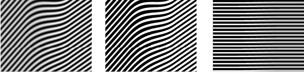
FIG. 5.4. Microstructure models for continuous vector fields m(x) = (m_1(x), m_2(x)) . Left to right: Amplitude-Angle, Volume Fraction-Angle, Amplitude-Volume Fraction.
