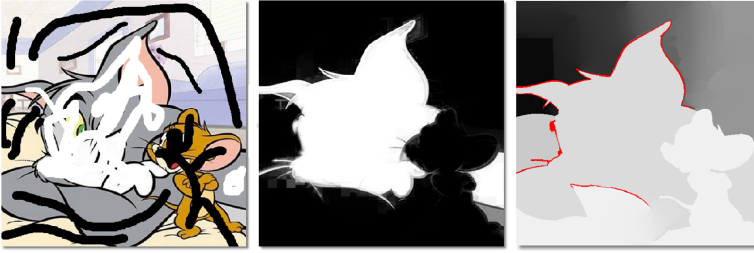
Figure 15: Image matting could improve the depth assignment. Left: user interaction; middle: \alpha matting result; right: refined depth maps (see the improvement on the red boundaries).
